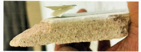
The photo above shows the use of drywall muds on gypsum plaster and the typical thickness of applications.
